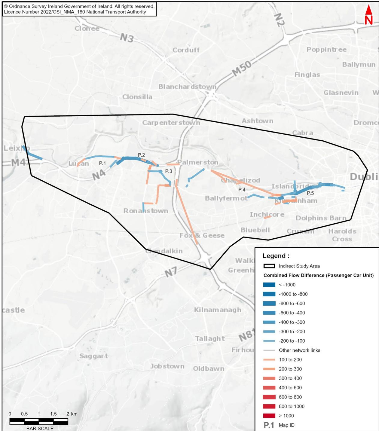
**Diagram 6.28: Flow Difference on Road Links (Do Minimum vs. Do Something), PM Peak Hour, 2028 Opening Year**
