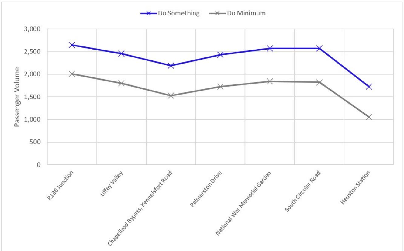
**Diagram 6.13: 2043 AM Peak Hour Passenger Volume Along Proposed Scheme (inbound direction)**
