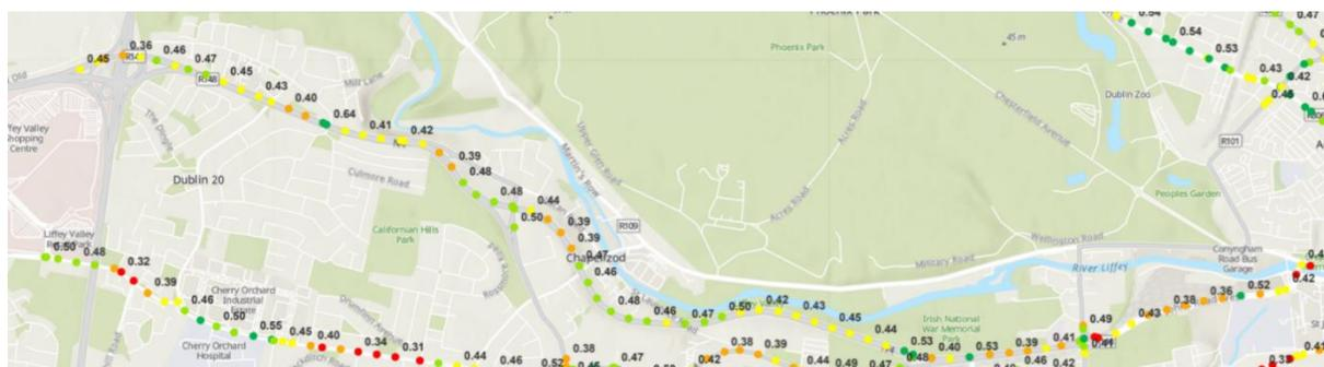
**Figure 7-4 Corrected SCRIM Conditions for Proposed Scheme (from M50 Jct. 7 to Heuston Station).** Source: ArcGIS RMO MapRoad (2019 DCC Pavement Surveys) - Esri UK, Esri, HERE, Garmin, METI/NASA, USGS mapping
