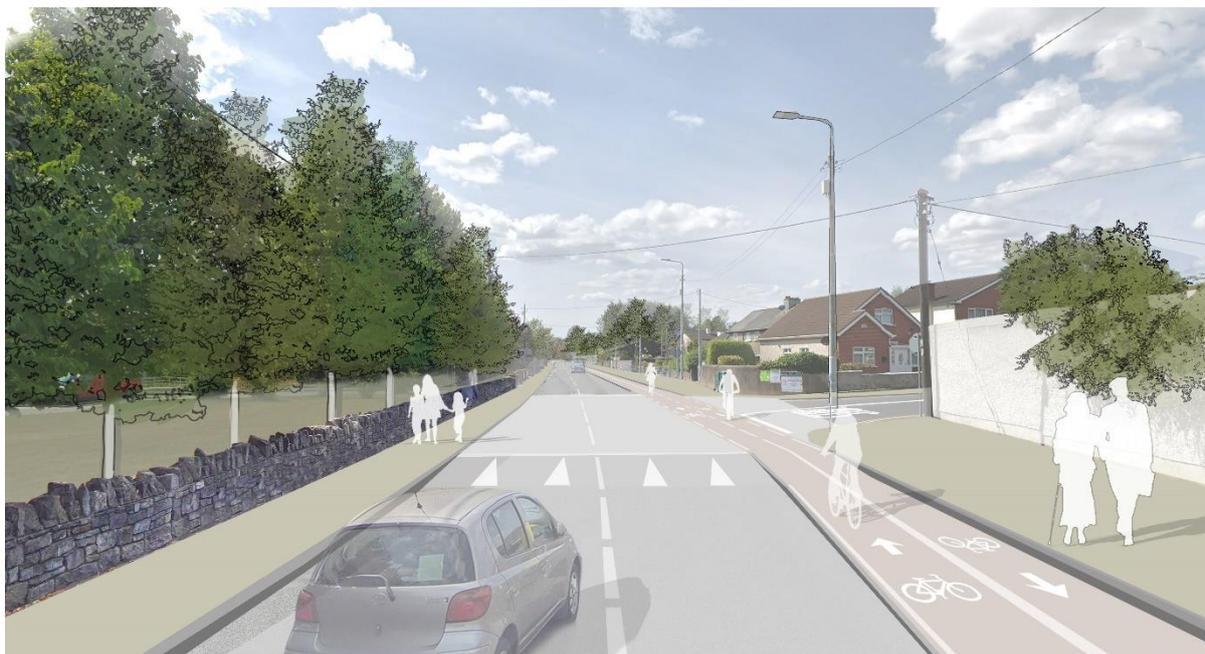
**Figure 14-10 Design Intent Sketch - Two-way Cycle Track Along the Full Length of Old Lucan Road by Reallocating Road Space**
